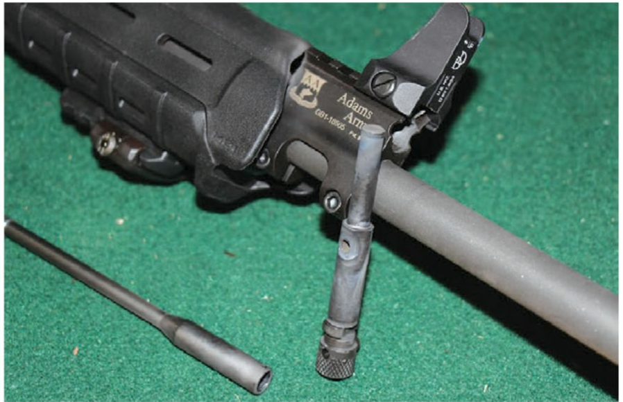
Piston removed from the gas block. This makes for easy maintenance. Gas block has a rail on top for a sight tower if you want back-up iron sights for your optic.
