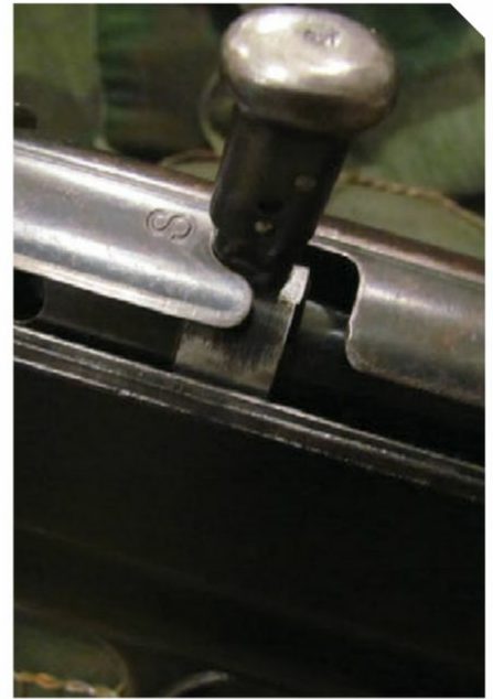
Primary safety on MP40 is bolt retention slot that locks bolt open to the rear.
