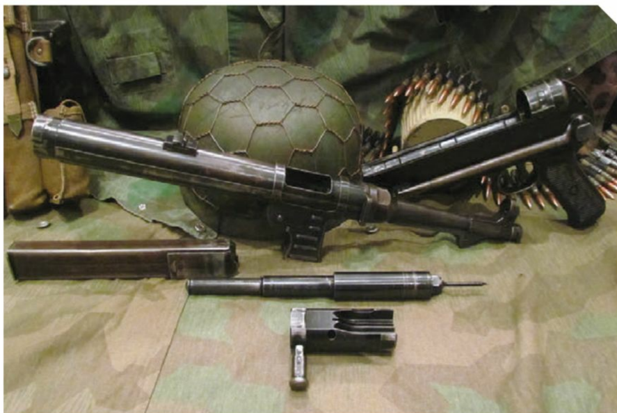
German MP40 is simple to maintain in the field. It breaks down into major subcomponents easily and without tools.
