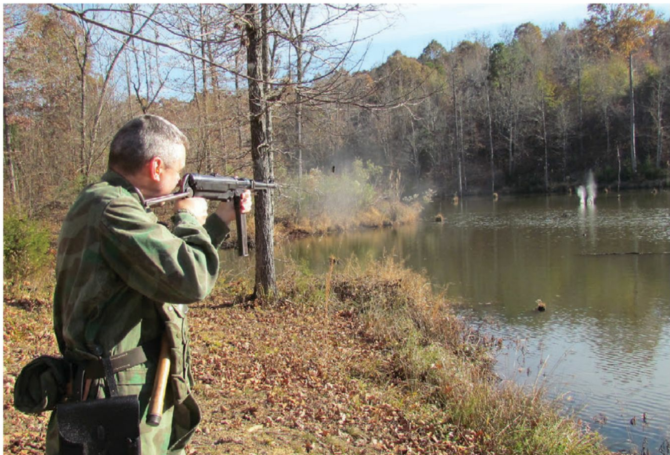
In action, German MP40 is eminently controllable. Gun's imposing weight, forward center of gravity, and light recoiling cartridge all conspire to defeat muzzle rise during long bursts.
