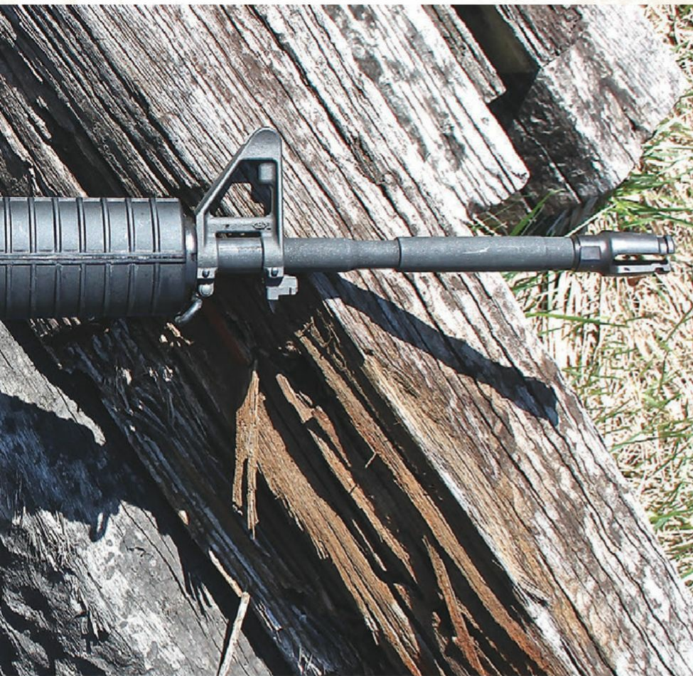
Standard A2 flash hider was replaced with Valmet-pattern VAL-76 three-prong flash hider.
