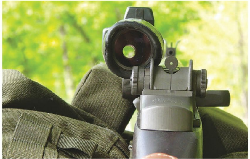
View from rear of offset scope, which allowed M1D to still be loaded with eight-round clips.
