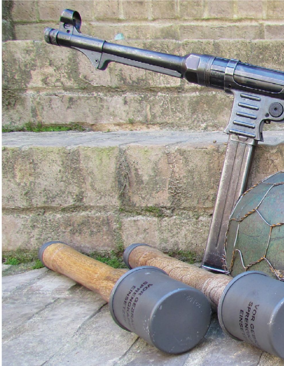
Above: MP40's hefty nine-pound weight, combined with its diminutive 9mm cartridge and sedate rate of fire, make for a controllable platform.
