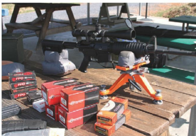
Leupold Mark 4 3.5-10X scope was mounted on C15 M4 for bench accuracy testing in conjunction with Champion tripod front rest and rear sandbags.
