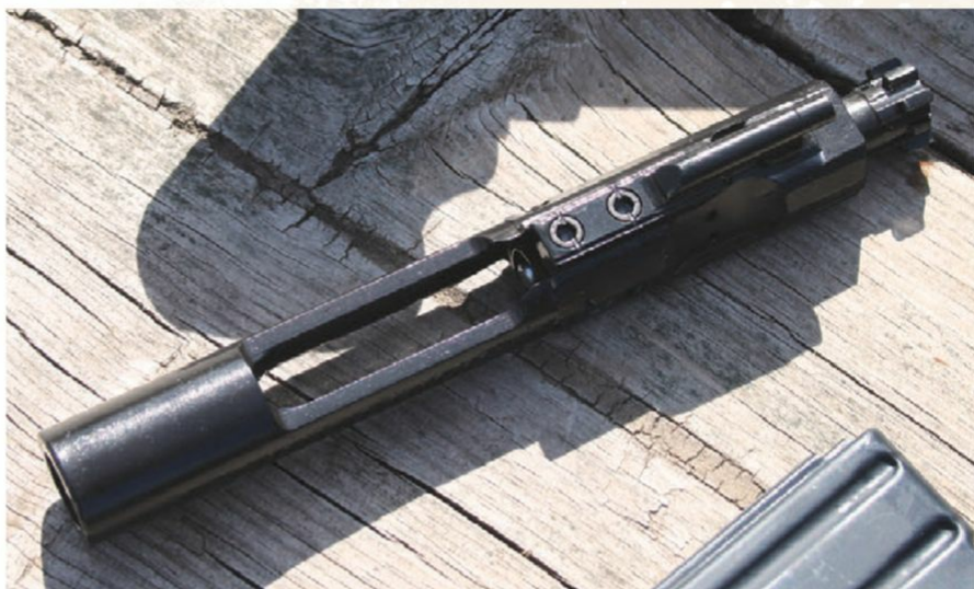
Above: Carrier key was properly staked.
