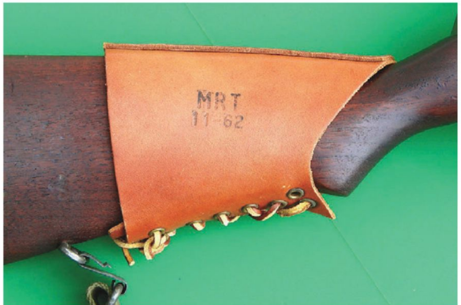
Right side view of cheek pad designed to position shooter's eye for use of offset scope on M1D.
