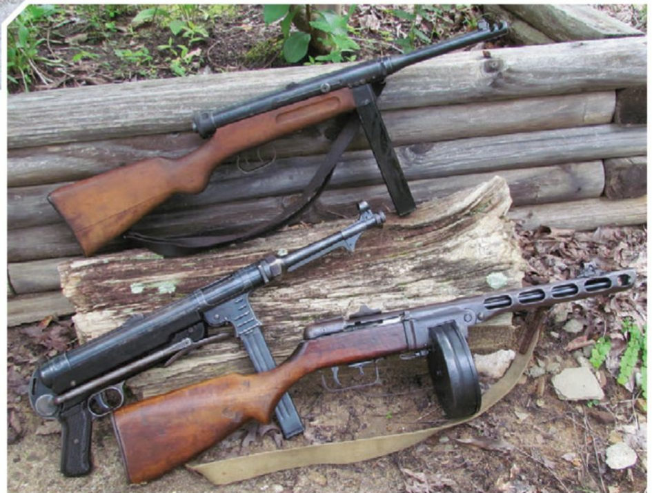
German MP40 (middle), Italian Beretta 38/42 (top), and Soviet PPSH (bottom) demonstrate various approaches to submachine gun design exhibited by some of major combatants during WWII.
