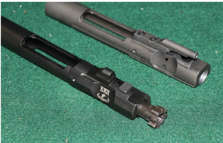
Front: Adams Arms bolt carrier and bolt. Rear: direct impingement bolt carrier. After 100 rounds, Adams Arms carrier is still as clean as when author put it in.
