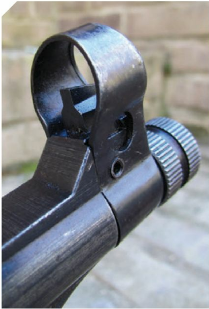
Front sight on MP40 is protected by a heavy hood.
